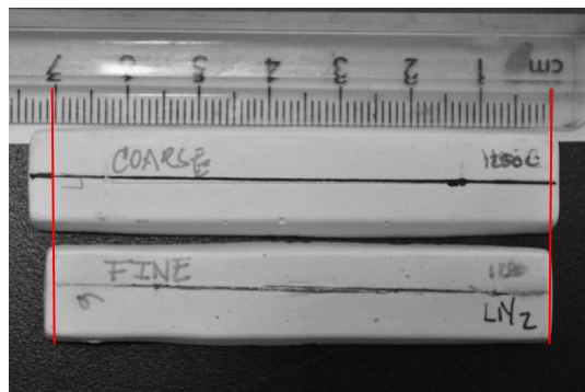
Figure 4.13: Coarse and fine powder samples fired at 1200°C
