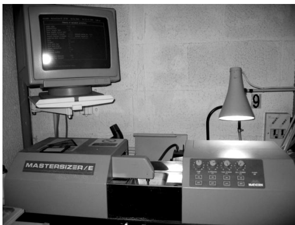
Figure 3.6: Mastersizer/E, International Manufacturing Centre University of Warwick.
