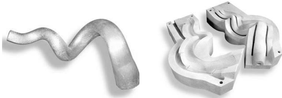
Figure 2.16: Cast metal part (left) produced from a z cast sand mould (right) Courtesy: Z corp U.S.A. [35]
