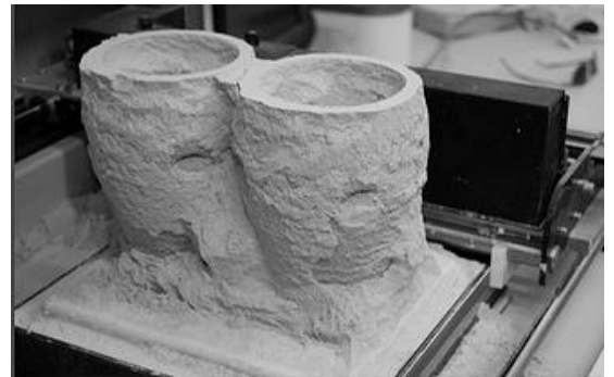
Figure 2.23: 3D printing of traditional ceramics powder, Bowling Green State University Ohio, USA.
