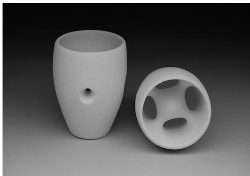
Figure 2.23: 3D printing of traditional ceramics powder, Bowling Green State University Ohio, USA.
