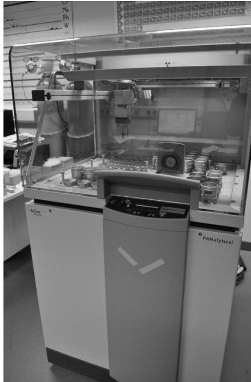
Figure 3.8: X-ray Fluorescence (XRF), Geology department, University of Leicester.
