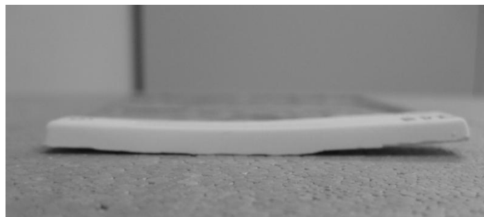
Figure 5.8: Pyroplastic deformation of the freeze-cast ceramic specimen fired at 1150°C
