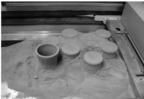
Figure 2.25: Printing Object on ceramic powder. Courtesy: the Solheim Rapid Manufacturing Laboratory. Mechanical Engineering Department at the University of Washington. Seattle [43]
