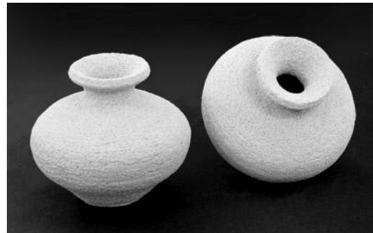
Figure 2.25: Printing Object on ceramic powder. Courtesy: the Solheim Rapid Manufacturing Laboratory. Mechanical Engineering Department at the University of Washington. Seattle [43]
