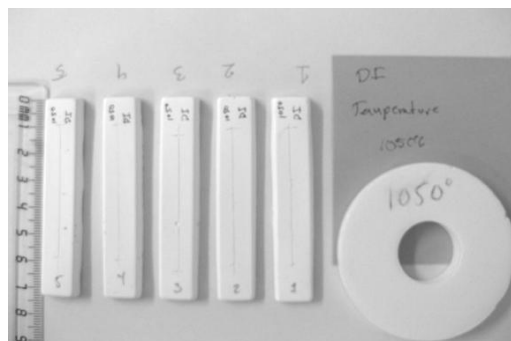
Figure 5.7: Freeze casting specimen bars after being fired at different temperatures
