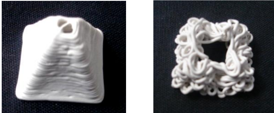
Figure 4.22 Flattening of layers due to insufficient stand-off (left) and curling of the bead due to excessive stand-off (right).
