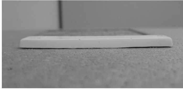
Figure 5.9: Freeze-cast ceramic specimen fired at 1075°C
