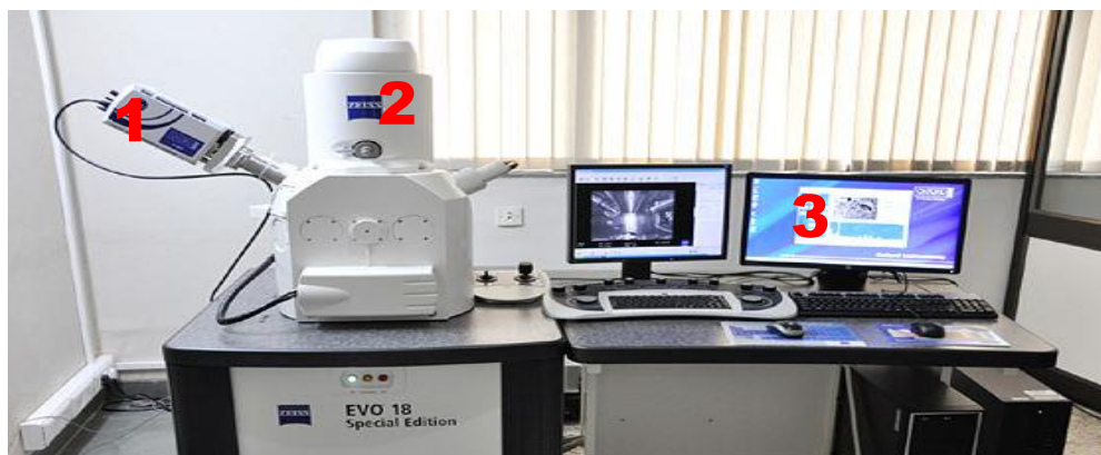
1: Energy Dispersive X ray spectroscope 2. Scanning electron microscope 3. Monitoring screen
