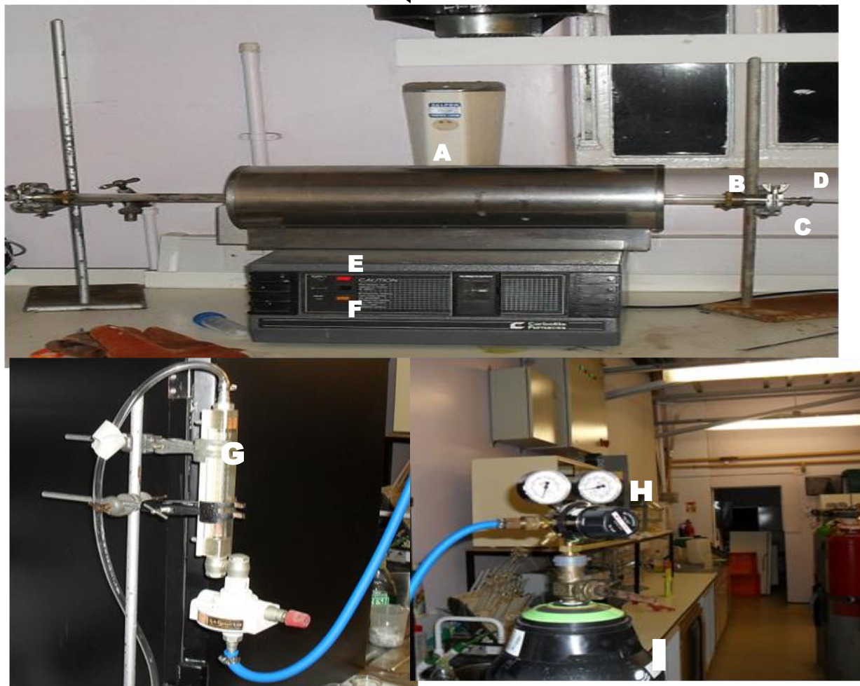
A: Carbolite furnace B: Quartz tube C: Cast clamps D: Parker A-Lok E: Power button F: Power indicator G: Flow meter H: Pressure gauge I: Nitrogen Cylinder
