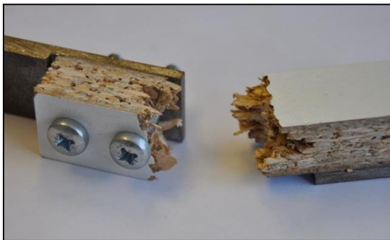
Figure 12.3 – An example of a test bracket failing
