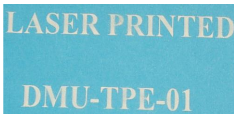
Figure 121 Laser printed Somos201(TPE)using HP LaserJet4
