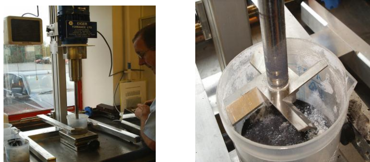
Figure 98(a) Lab scale mixer & (b) Paddle type mixing blade
