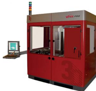
Figure 1a) Bench-top machine developed by Hull and (b) Commercial SLA machine
