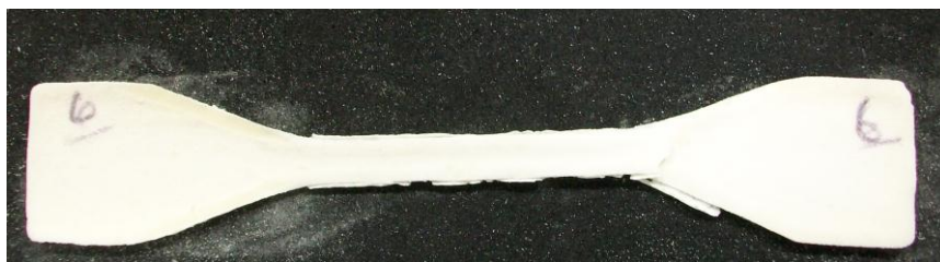
Figure 176 uncoated 17 \mu\text{m} particle size sintered for 60 seconds under IR radiation
