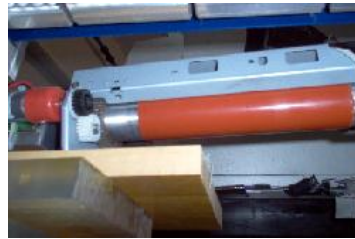
Figure 83 Heated levelling roller for Test Rig
