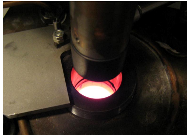
Figure 73(a) Demonstration Test rig MPP & (b) Sintering die
