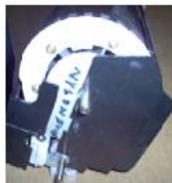
Figure 88 standard transfer roller fitted with Nylon bush (non-conductive) around the main shaft
