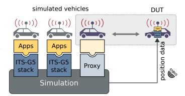
Fig. 1. Simulation and DUT testbed
