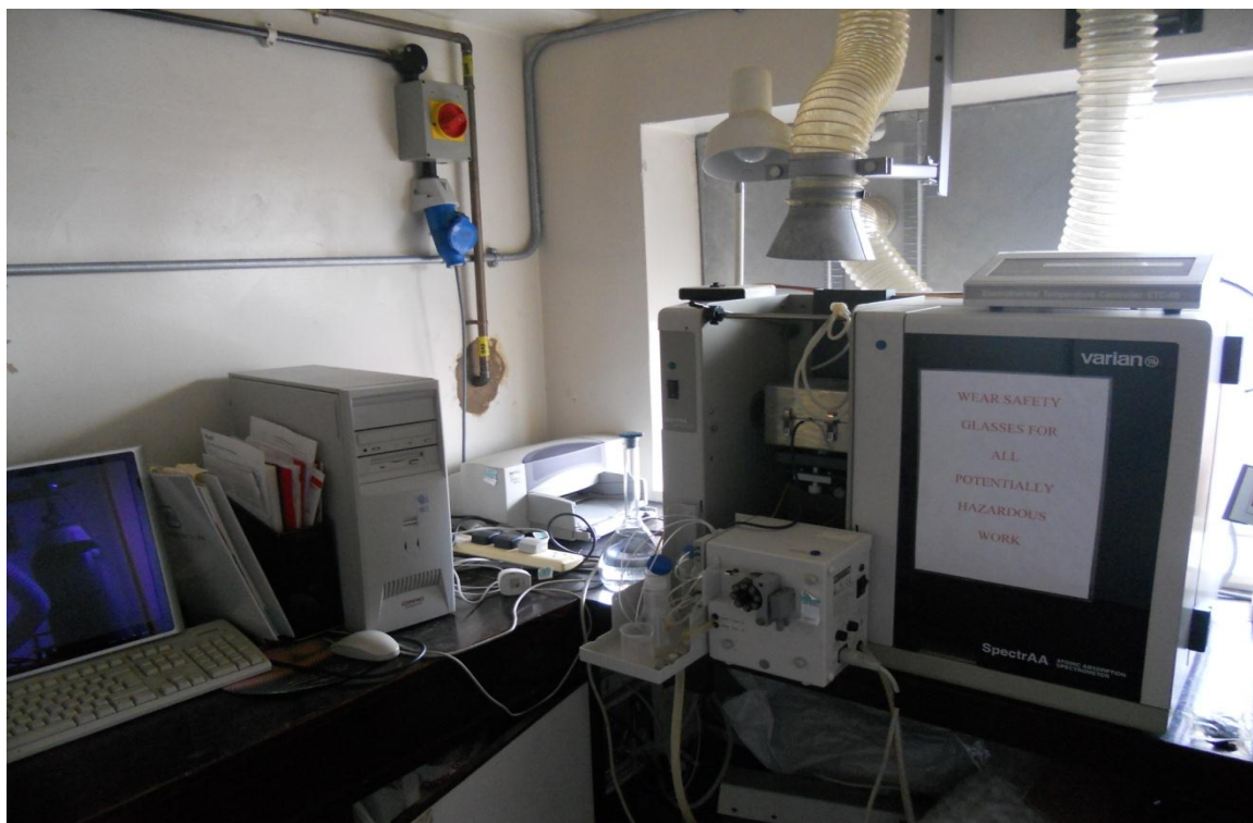
Figure 2.5: Graphite furnace atomic absorption spectrometry (Varian model 220-Z), GF- and HG-AAS.
