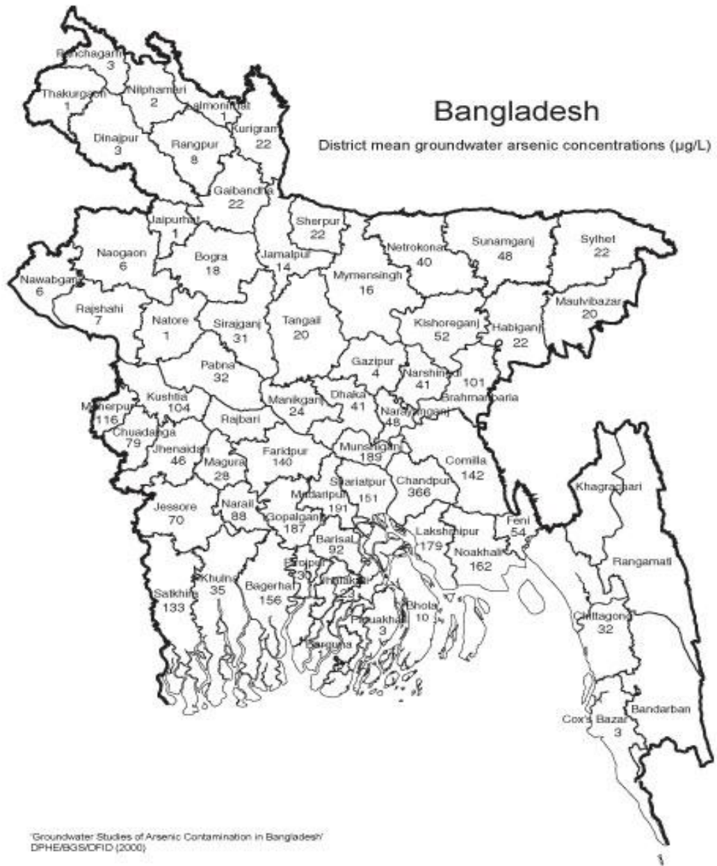
Figure 3.1: Arsenic levels in groundwater in different districts of Bangladesh. Source of diagram: British Geological Survey (BGS, 2011).
