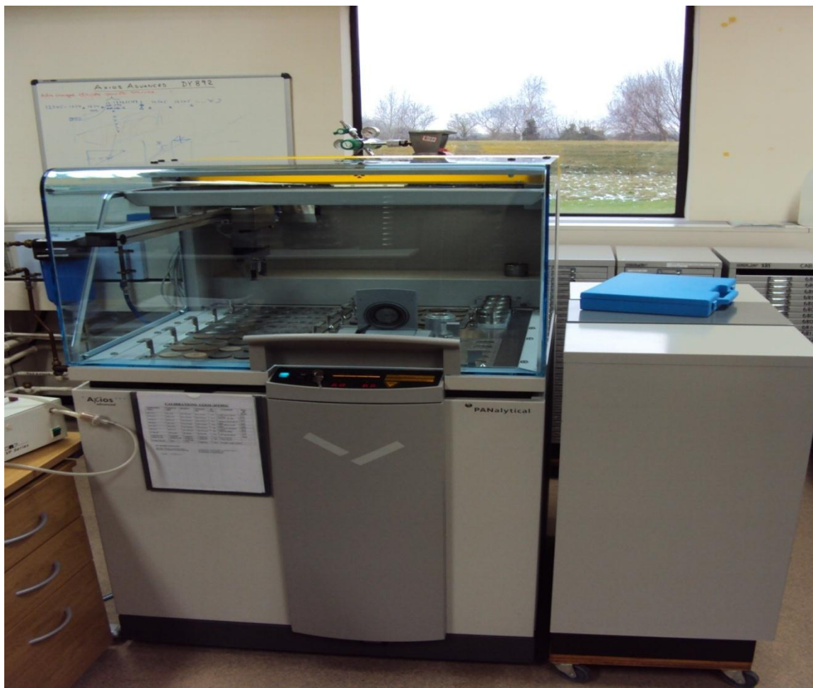
Figure 2.8: Energy dispersive X-Ray Fluorescence Spectrometry (XRFS) (PANalytical Axios advanced WD-XRFS).
