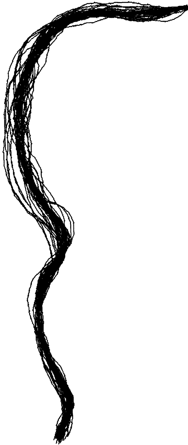
Fig. D.10. The Tracked Paths of the Geometric Type-2 Robot FLC.
