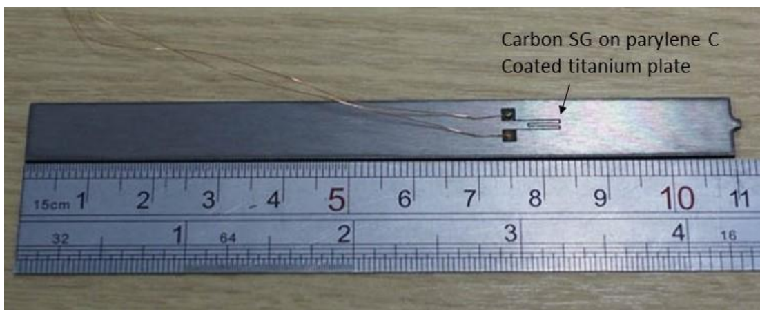
Figure 9.13 MDDW carbon strain gauge on parylene C coated titanium test-plate
