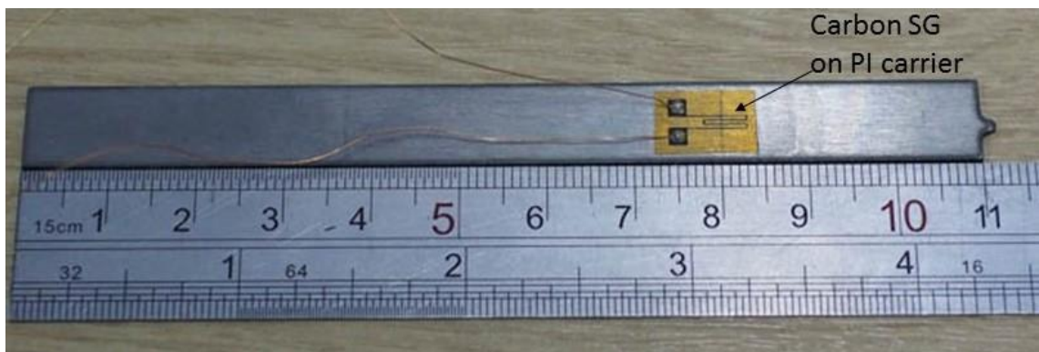
Figure 9.10 Image of a carbon resistive strain gauge sample on titanium test-plate
