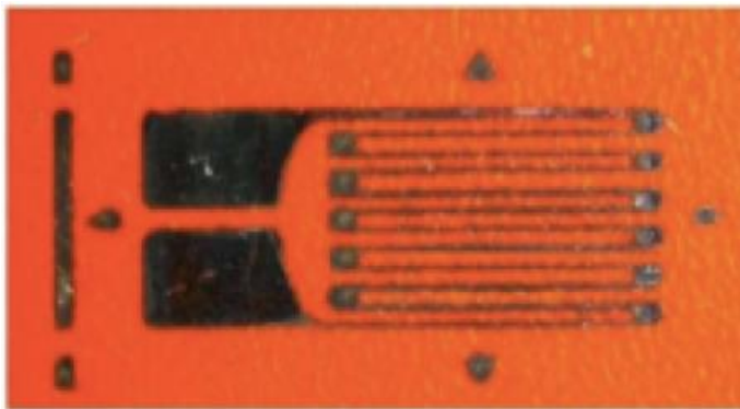
Figure 5.12 Silver strain gauge fabricated with DOD ink-jet printing on polyimide film [94]
