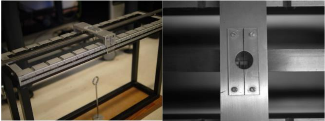
Figure 7.19 Mechanical test of silver strain gauge using three-point measurement
