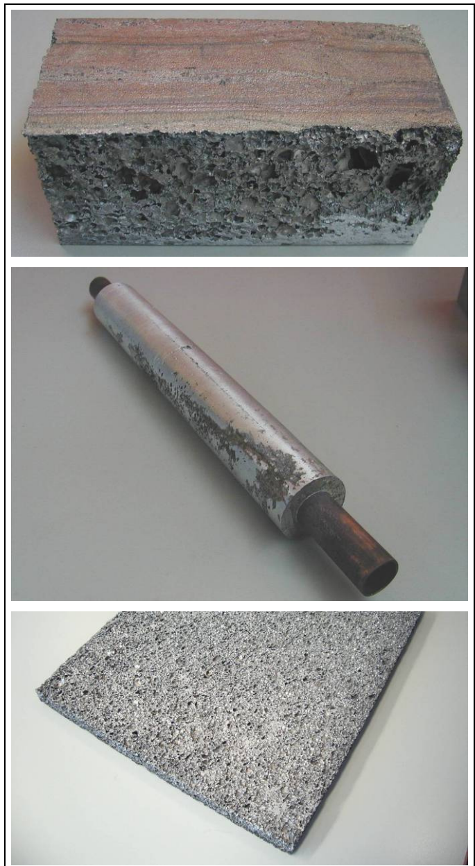
Figure 3.30: Open Cell Aluminium Foam Samples
