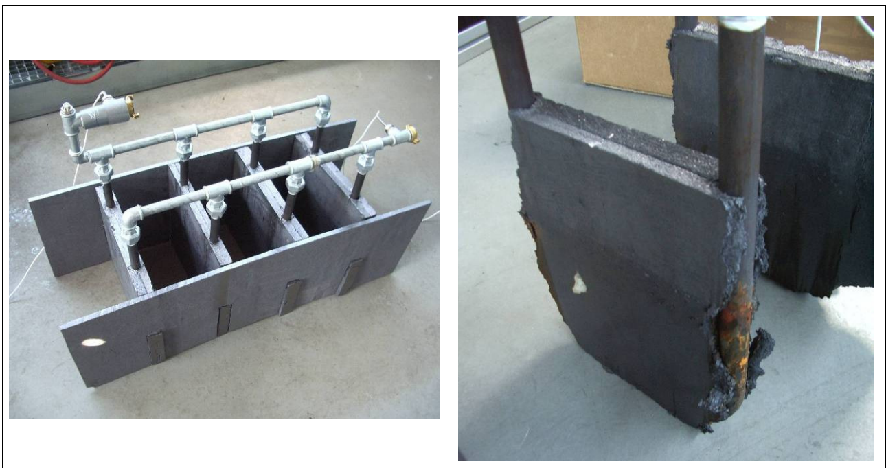
Figure 3.32: Heat Exchanger with Expanded Graphite as Heat Conduction Matrix
