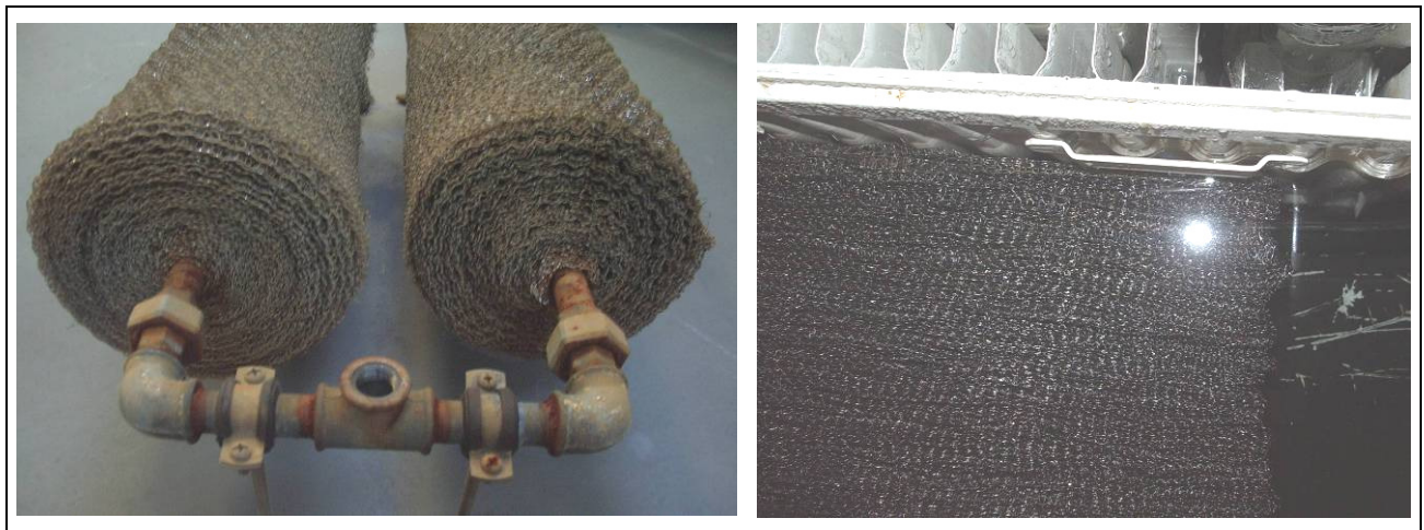
Figure 3.33 : Heat Exchangers with Wire Netting as Heat Conduction Matrix
