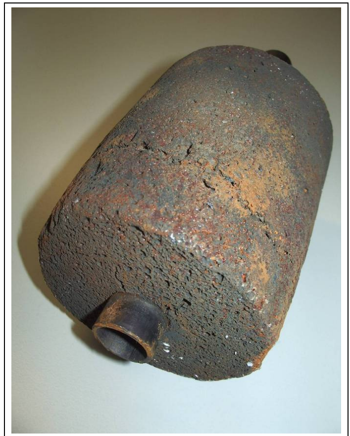
Figure 3.31: Steel Foam Sample (length: 110mm, diameter: 90mm)
