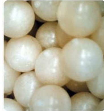
Figure 3.16: Spherical Nodules containing PCM, poured in a Storage Tank [89]
