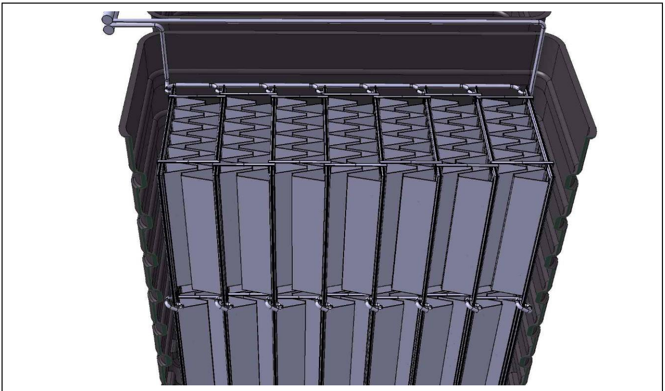
Figure 3.43: Interior View on the Heat Exchanger Arrangement inside the Storage Tanks
