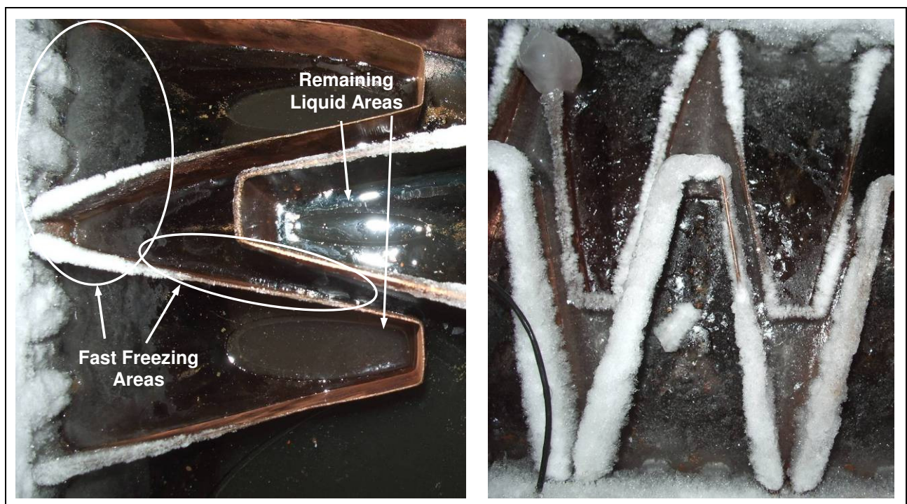
Figure 3.37: Behaviour of Sheet Matrix Heat Exchanger, during freezing (left) and completely frozen (right)
