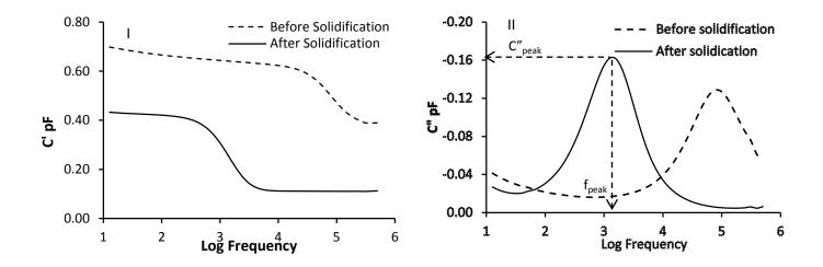
**Figure 2** Capacitance plots during the freezing of a sucrose solution (30 mg/ml) (I) left shows the frequency dependence of the real part of capacitance (C') and (II) right shows the frequency dependence of the imaginary part of capacitance (C") The dotted line represents liquid state and the solid line denotes frozen state.
