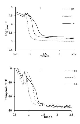
**Figure 4**. Time profiles of (I)  $f_{peak}$  and (II) temperature for 30mg/ml sucrose during freezing at different fill factors ( $\phi$  =0.5, 1 and 1.6). (n = 10) Note that time zero is taken from the end of the equilibration phase after the vial and contents have been equilibrated at 25 °C for 10 min.
