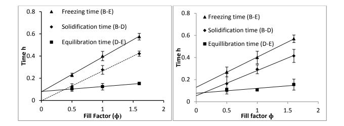
**Figure** 6 Freezing time, solidification time and equilibration time for 3% w/w sucrose solution at different fill factors (n = 10), (LEFT) Impedance measurement (RIGHT) Thermocouple measurement.
