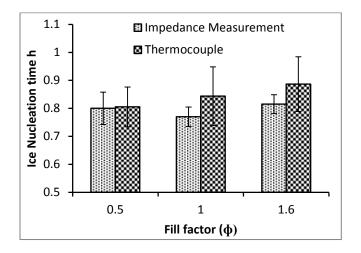
**Figure 5** Ice nucleation time for sucrose 30mg/ml at different fill factors. Time zero is taken from the end of the equilibration phase after the vial and contents have been equilibrated at 25 °C for 10 min. The nucleation time is then calculated from the time point B (Fig. 3).
