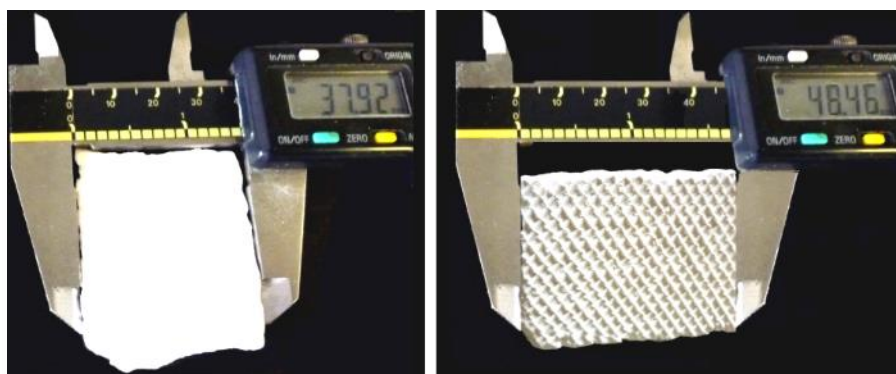
Figure 88: Photographs of an 85% SF Ribbon composed of 78.6 % MCC, 19.4 % Lactose anhydrate, 1½ croscarmellose and ¼ % Mg St.
