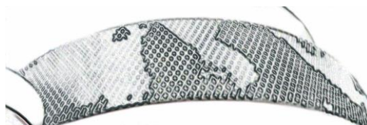
Figure 84: Enhanced photograph of a knurled roll-wheel following ~20 minutes of operation of a Gerteis PolyGran with a multi-component placebo ‘typical blend’ 27 .
