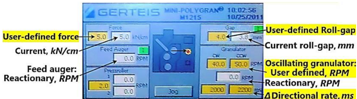
Figure 79: Labelled photograph of the Gerteis PolyGran GUI. The yellow fields are set by the user and the corresponding white fields are the real-time system responses.
