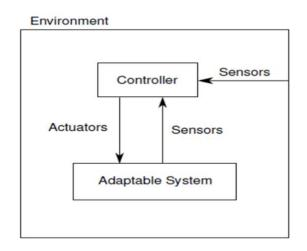
Figure 2.5: Adaptive System Architecture [82]
