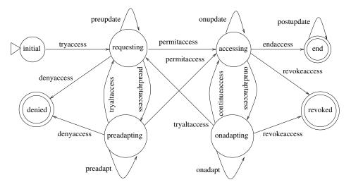
Figure 3.2: Execution of an access request in the CA-UCON model
