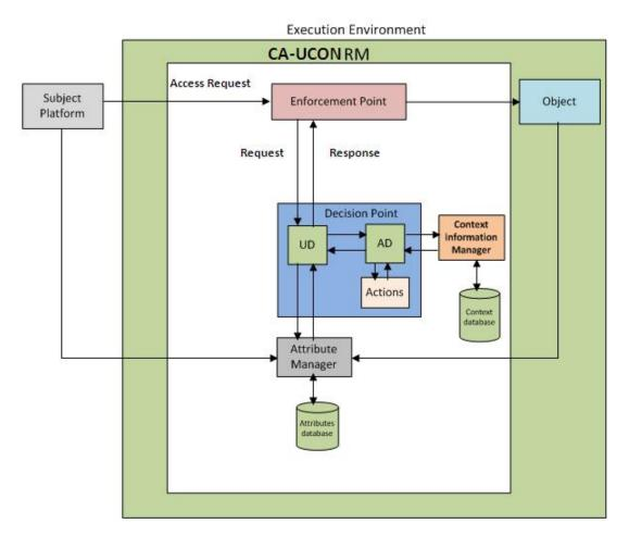
Figure 6.1: Architecture of the CA-UCON Reference Monitor
