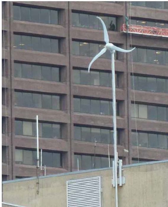
(b) An HAWT mounted on the side of the Boston Museum of Science [Smith et al., 2012].
