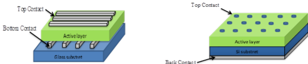
Figure 4.1 Illustration of (a) MIM devices (b) MIS structure (Metal-insulator-blend-semiconductor).
