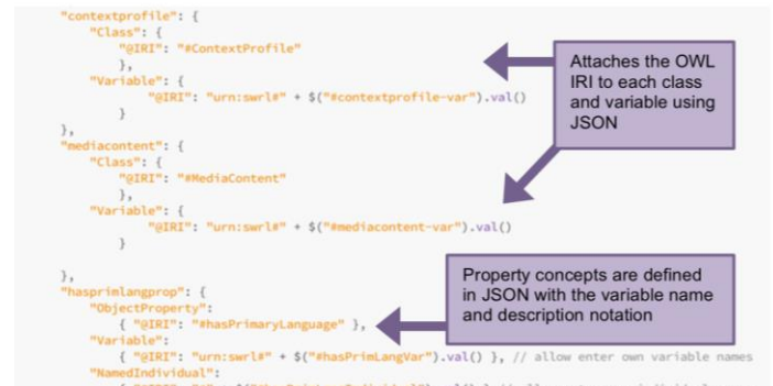
Fig. 7-Fig. 9. Snippet of JSON notation used to create the ontology classes and properties. Each JSON object contains the class or property name and associated variables.
