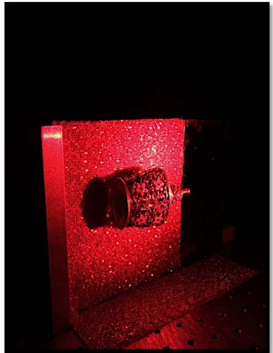
Figure 4.66 Photograph of the object to record the transmission hologram with red laser beam before shooting
