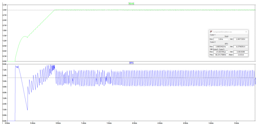
Figure 12: Simulated Output Voltage of 3V, Load Current of 6A
