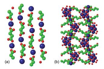
**Fig. 1** Structures of cobalt succinate: (a) phase A and (b) phase F. Larger (blue) spheres represent cobalt ions; medium (green) spheres represent carbon, smaller (red) spheres oxygen. Hydrogen atoms and water molecules have been omitted for clarity.
