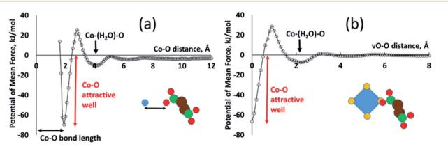
Fig. 3 PMF for the interaction of Co<sup>2+</sup> ion and carboxylate O species (a) and its re-interpretation within our virtual-site coordination model as the equivalent interaction of vO and O (b), with a zero vO-O distance in the attractive well, and with the long-distance average value of the PMF shifted to zero.
