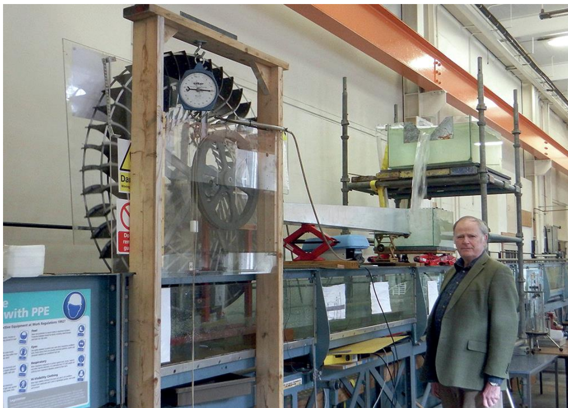
Figure 7. Test set-up at Abertay University (Picture annotation to show: Kelvin dynamometer, V-notch weir, Level flume, Stilling tank)
