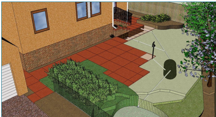
Figure 4 Stormwater management train for a house-plot: roof water is attenuated in an underground rainwater harvesting tank, with overflow to natural rain garden. The driveway uses permeable paving.
