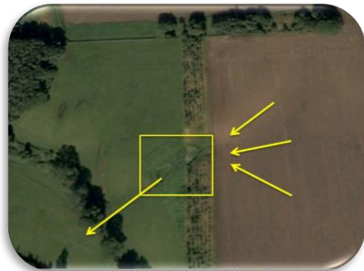
Location showing arable field, buffer strip, Sediment Trap Bund and Pond and the exceedance (extreme rainfall event) overland flow route to watercourse
