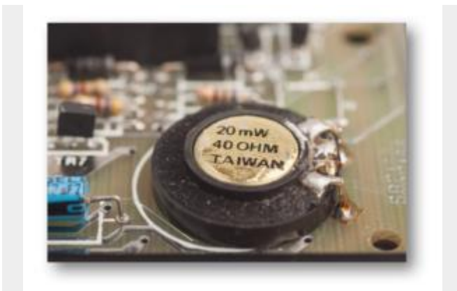
Figure 3: The 22mm speaker from a 1983 Issue 4B Sinclair ZX Spectrum, which provided a single channel of 1-bit sound.
