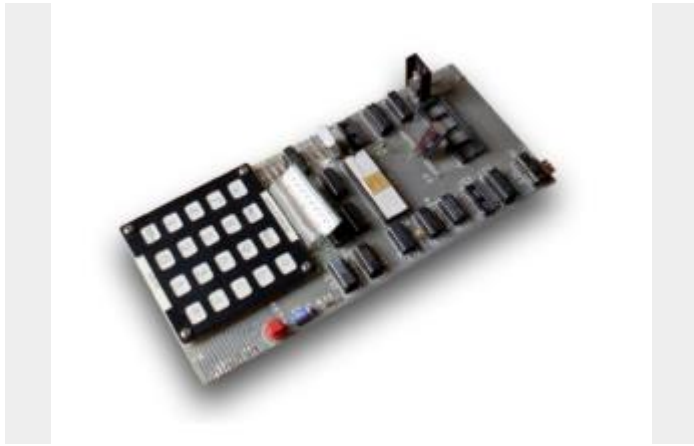
Figure 1: The Science of Cambridge MK14 has a form factor and interface that shows a clear lineage from the company's handheld LED calculators, and was an important first step in the development of mass home computing.
