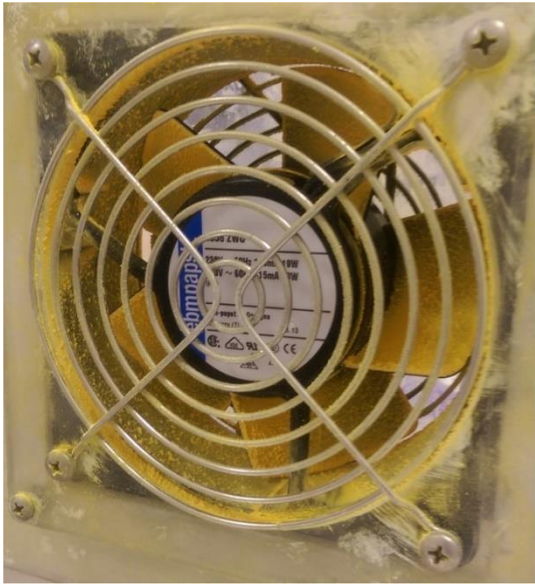
Figure 11 - PECA Multiband powder residue problems in fuming cabinet components
