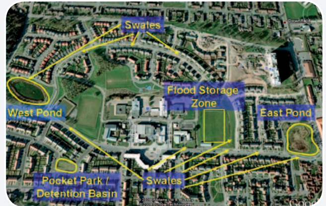
Figure 1 SuDS in Ardler Village, Dundee, Scotland. Source: image by kind permission of Alison Duffy, UWTC, University of Abertay Dundee. Based on Google map © 2009 Infoterra Ltd & Bluesky, © 2009 Europa Technologies, © 2009 Tele Atlas.
