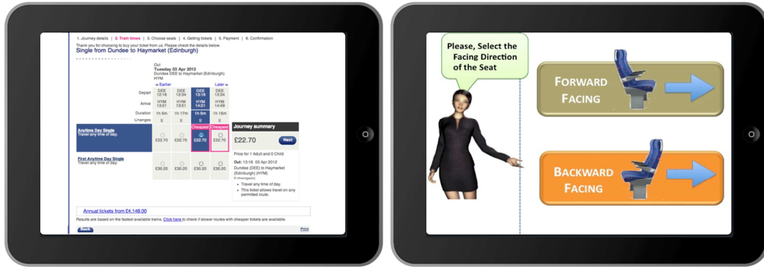
Fig. 4 Screenshot of the interfaces for the train ticket transaction. (a) On the left, the web interface. (b) On the right, the equivalent UI built according to the recommendations given for designing for an OU.
