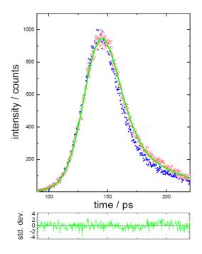
**Figure 6.** Representation of the decay of lycopene in hexane (red), also showing the IRF (of 36 ps—blue), fitted function (2 exponential green) and weighted residuals (green), close to the peak of the decay. The excitation wavelength was 409 nm (DD-405L) and the emission at 550 nm. Adapted from [48].
