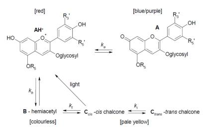
Scheme 2. Relationship between the different anthocyanin (AH<sup>+</sup>, A, B, Ccis, Ctrans) forms adapted from [100] and [colour] indications from [99].
