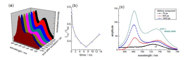
**Figure 3.** TRES measurement performed on a whole leaf (*Ficus*), showing (**a**) time-resolved emission spectra; (**b**) change in peak ratio of the principal emission bands with time after excitation and (**c**) decay associated spectra obtained via a global analysis of the TRES dataset. Adapted from [45].
