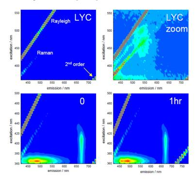
**Figure 4.** Fluorescence excitation-emission spectra (EEM's) for the samples, showing excitation wavelength (*y*-axis) emission wavelength (*x*-axis) and the intensity as rainbow scale (red—high, blue—low). The lycopene EEM (LYC) has also been scaled (LYC zoom) to show the lower intensity emission at ~550 nm. The scattering positions relating to Rayleigh, Raman and second order are also indicated. Adapted from [48].
