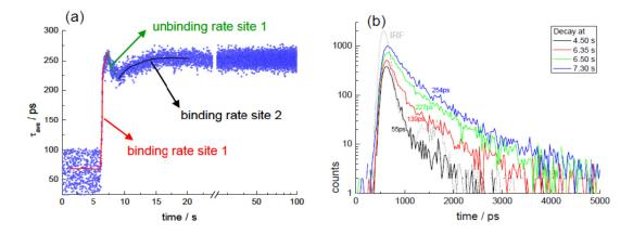
**Figure 12.** Binding of turmeric extract with serum albumin; (**a**) outcome of a two exponential analysis from a kinetic TSCPC dataset. 10,000 decay histograms were collected, each with an acquisition time of 10 ms; (**b**) representative decay histograms at different times at the beginning of the binding process. Adapted from [44].
