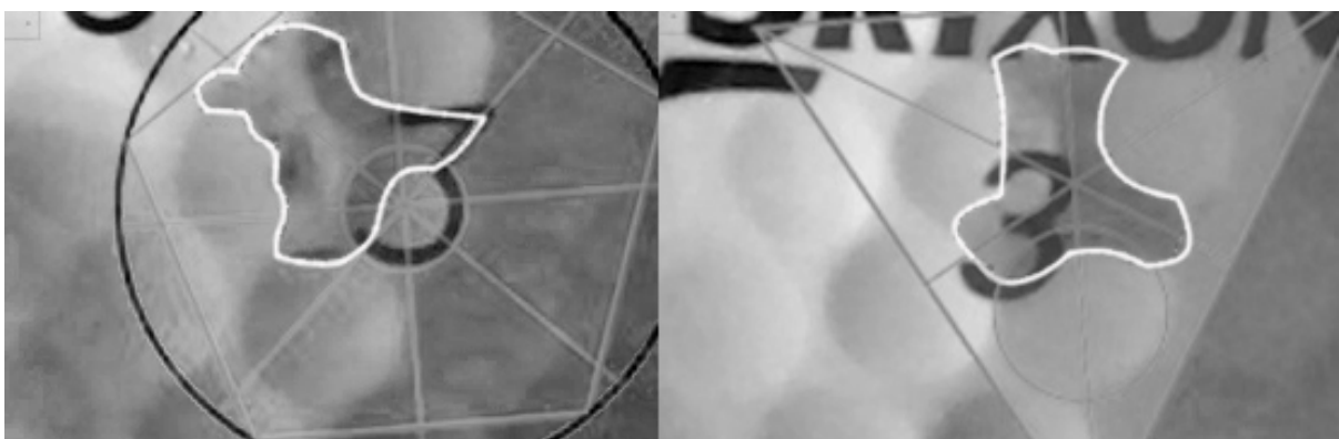
431 Figure 2. Step by step process of constructing and intersecting a polygon to identify 432 the coordinate of the impact point.
