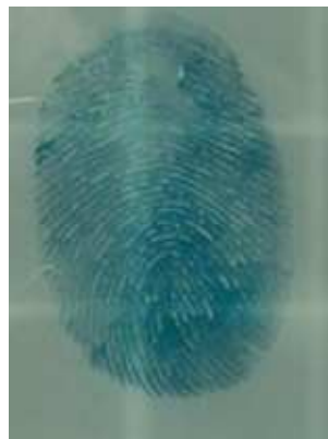
Figure 3: Enhancement of a fingerprint in blood on a plastic bag without the use of alginate with AB1 (28 days, no. 7 in the series)
