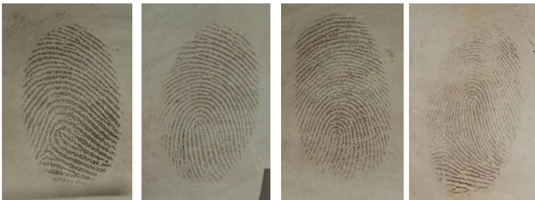
Figure 9 - Fingermarks developed with black magnetic powder on goshawk eggs after ageing: (a) 1 day; (b) 3 days; (c) 7 days; (d) 14 days
