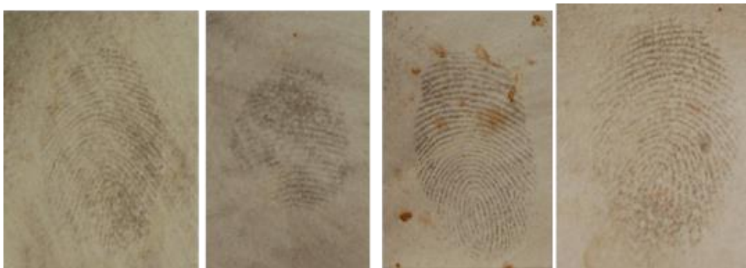
Figure 10 - Fingermarks developed with black magnetic powder on eagle eggs after ageing: (a) 1 day; (b) 3 days; (c) 7 days; (d) 14 days
