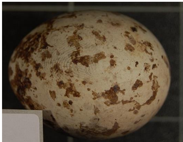
Figure 3 – Photography of a Sparrowhawk egg showing a developed fingermark with black magnetic powder.
