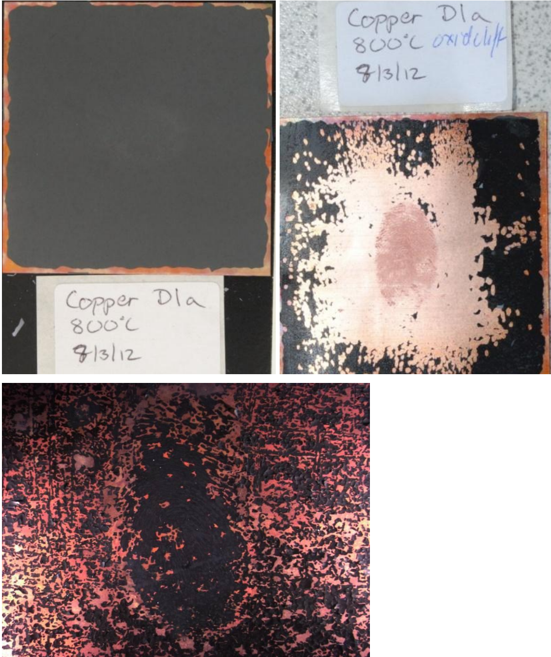
Figure 9: Copper heated at 800 °C for 5 min a) before lift showing slight evidence of fingermark, b) after oxide lift showing fingermark on underlying metal, c) copper heated to 600.
