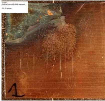
Figure 11 Fingermark on copper treated with 10-fold dilution of ammonium sulphide solution
