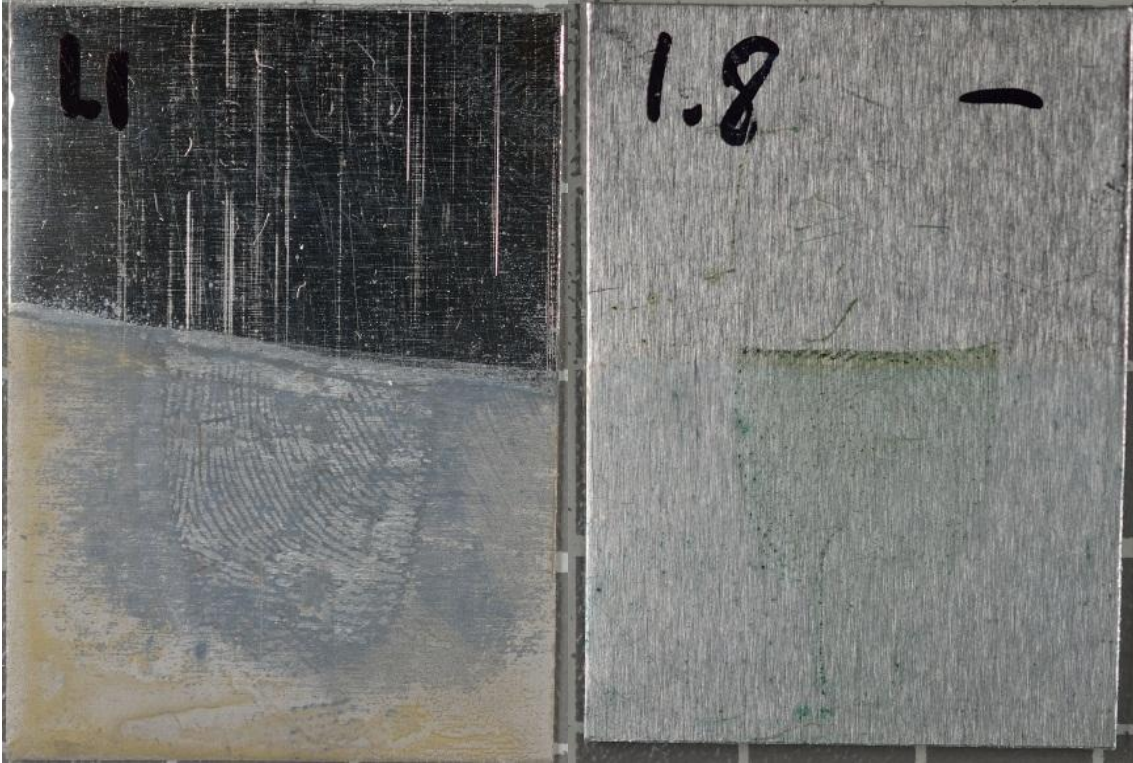
Figure 14 Anodised metal samples: a) fingerprint on tinned steel, and b) aluminium treated with anodising dye. Fingerprint marks were half submerged during processing to differentiate treated and untreated marks.
