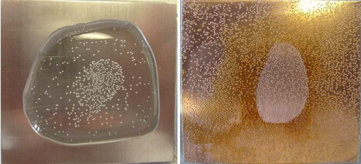
Figure 13 Fingermarks on copper: a) hydrogen peroxide solution, and b) carbamide peroxide solution with eccrine mark on the left and sebaceous-loaded mark on the right
