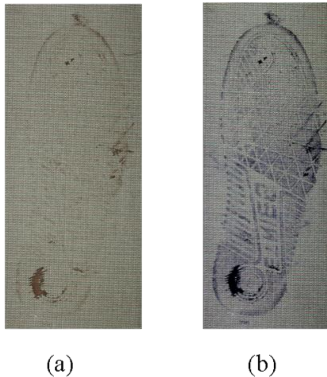
Figure 10 - Enhancement of a footwear impression in blood on patterned cotton using ninhydrin: (a) before; (b) after
