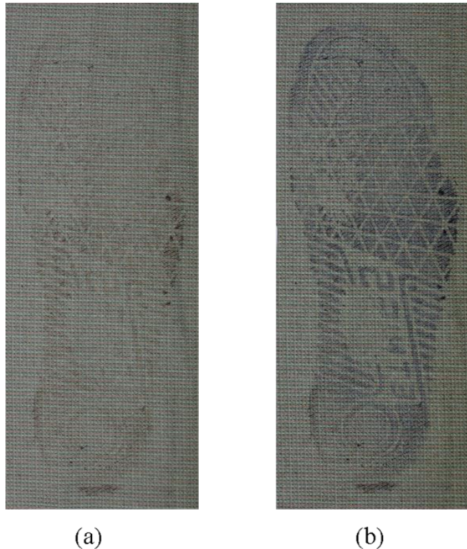
Figure 5 – LCV enhancement of a footwear impression in blood on patterned fabric: (a) before; (b) after
