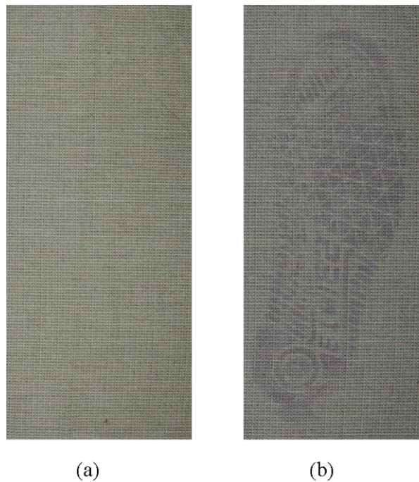
Figure 13 –Ninhydrin enhancement of a footwear impression in urine on patterned cotton: (a) before; (b) after
