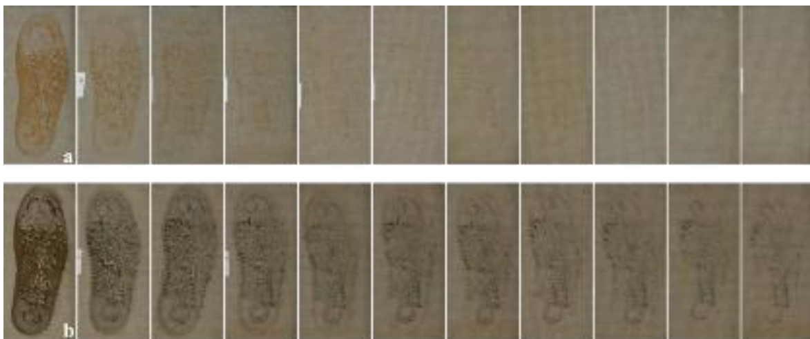
Figure 17 - Chemical enhancement of a diminishing series of footwear impressions in mud, prepared with Wemyss Bay (UK) soil on patterned cotton, with APD: (a) before; and (b) after enhancement
