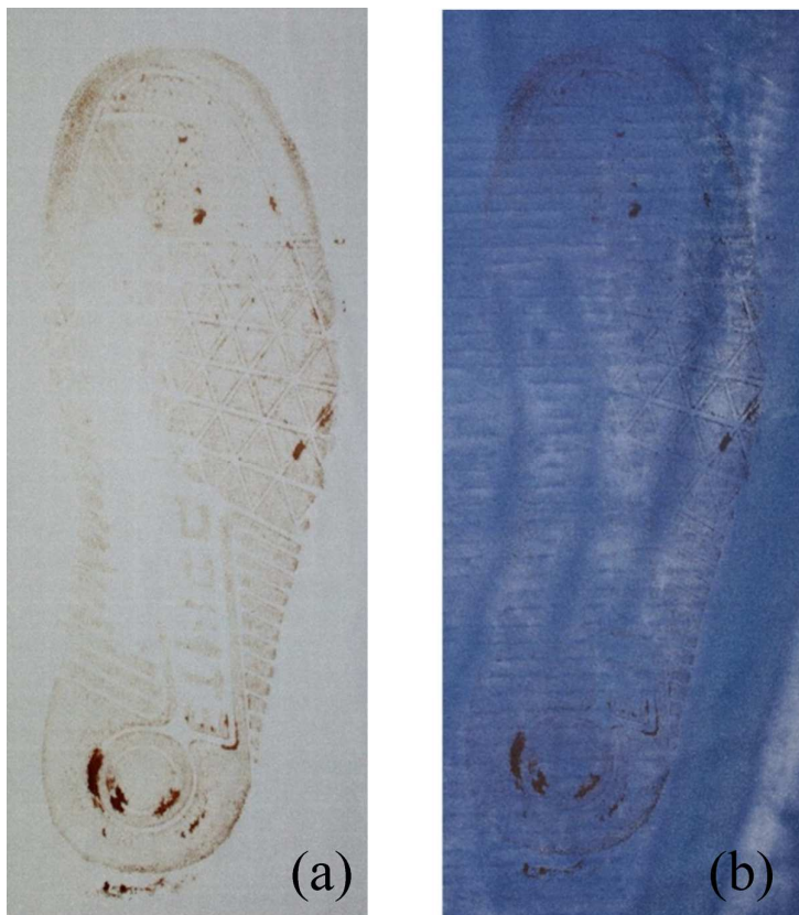
Figure 3 - Enhancement of a footwear impression in blood on white nylon/lycra using ninhydrin: (a) before; (b) after
