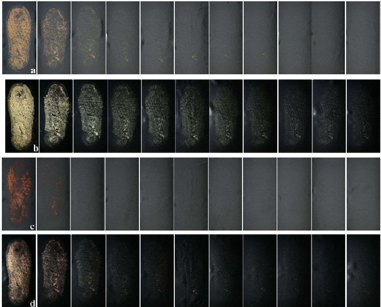
Figure 3 – Chemical enhancement of a diminishing series of footwear impressions in mud, prepared with Wemyss Bay soil on black polyester, with potassium thiocyanate: (a) 1 week old diminishing series; (b) observation with oblique lighting only; (c) enhancement with potassium thiocyanate; (d) enhanced diminishing series observed with oblique lighting
