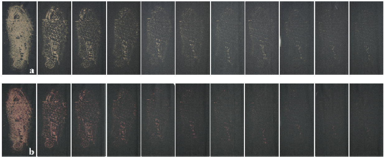
Figure 15 – Chemical enhancement of a diminishing series of footwear impressions in mud, prepared with the road soil sample on black nylon/lycra, with 2,2'-dipyridil: (a) before; and (b) after enhancement
