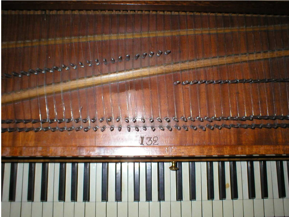
Figure 1 – Warping and cracking of the Kirckman’s soundboard. The main damage can be seen up and to the left of the serial number, below the nut.
