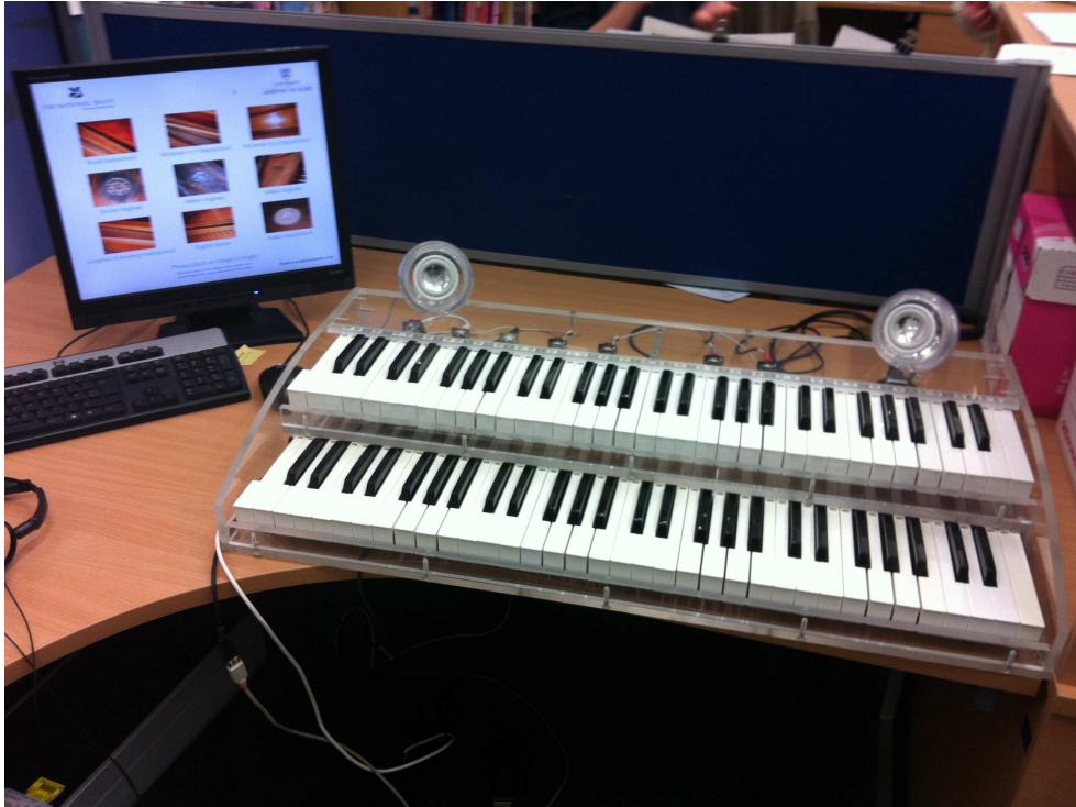
Figure 2 – The two-manual MIDI interface for the digital harpsichord.
