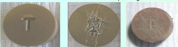
Fig 1. Original mark Fig 2. Defaced mark Fig 3. Recovered mark
