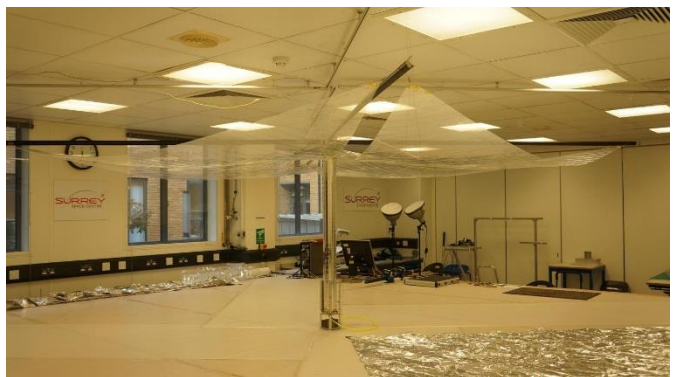
Figure 32: Dragsail: Deployment Test. With EQM unit.
