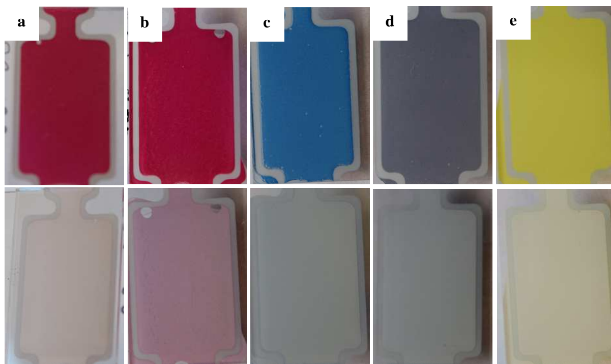
Figure 5: Out-of-plane electrophoresis test cell images of magenta particles synthesised by three-stage dispersion polymerisation in \text{scCO}_2 (a) and magenta, cyan, yellow and black by analogous synthesis in dodecane (b, c, d and e, respectively). The coloured state is shown above and the white state (from \text{TiO}_2 particles) below.
