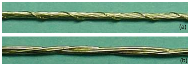
Figure 3 Steel cords (a) 12X; (b) 3X2
