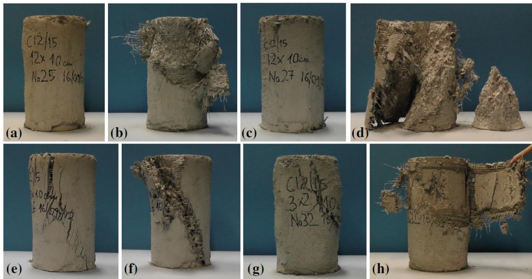
Figure 12: SRG jacketed cylinders at failure due to tensile fracture of the steel cords of the fabric: (a), (c), (e), (g) specimens at the end of the test; (b), (d), (f), (h) specimens after removal of loose mortar and concrete fragments.
