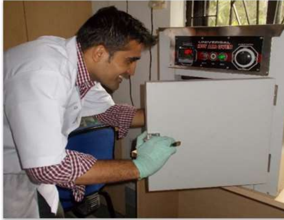
Figure 3.6: Hot air oven for determination of moisture content
