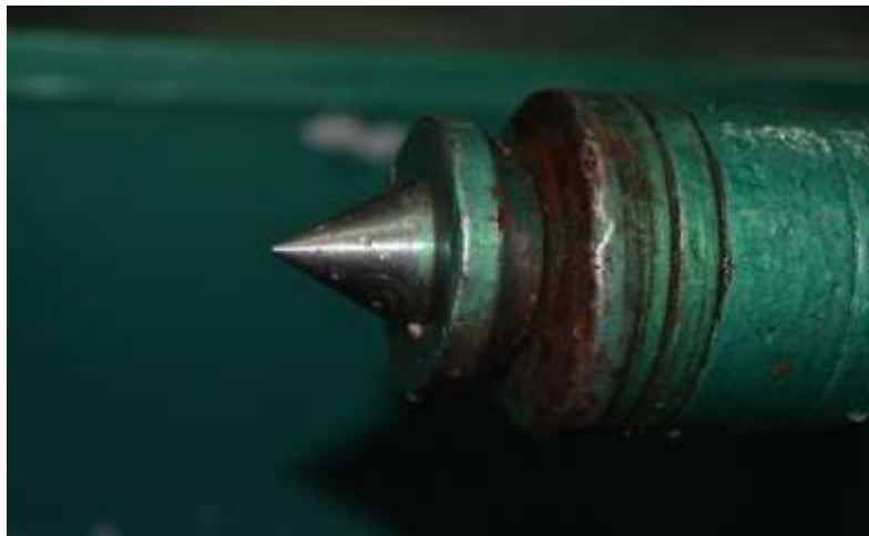
Fig 5: Driven end of holding assembly
