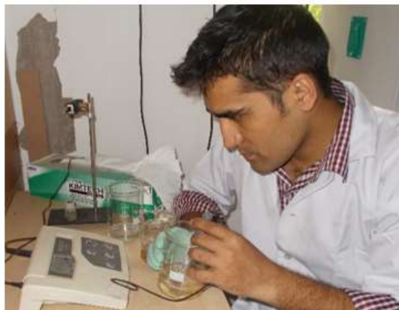
Figure 3.7: Determination of pH using pH-meter
