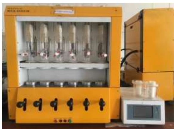
Figure 3.9: Socplus extraction system
