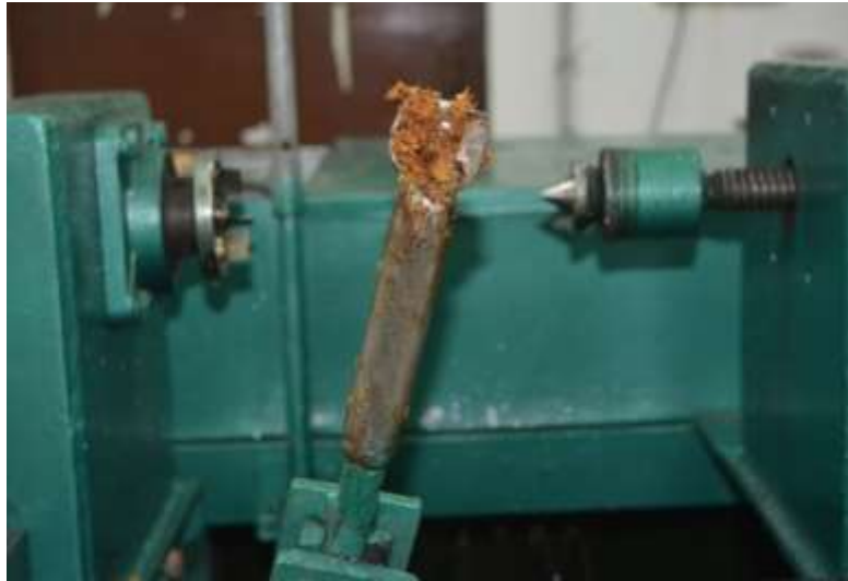
Fig 3: Jackfruit peeling blade and holding assembly.
