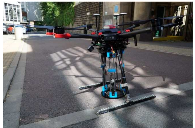
Fig. 2 Asphalt 3D Printing Drone.
