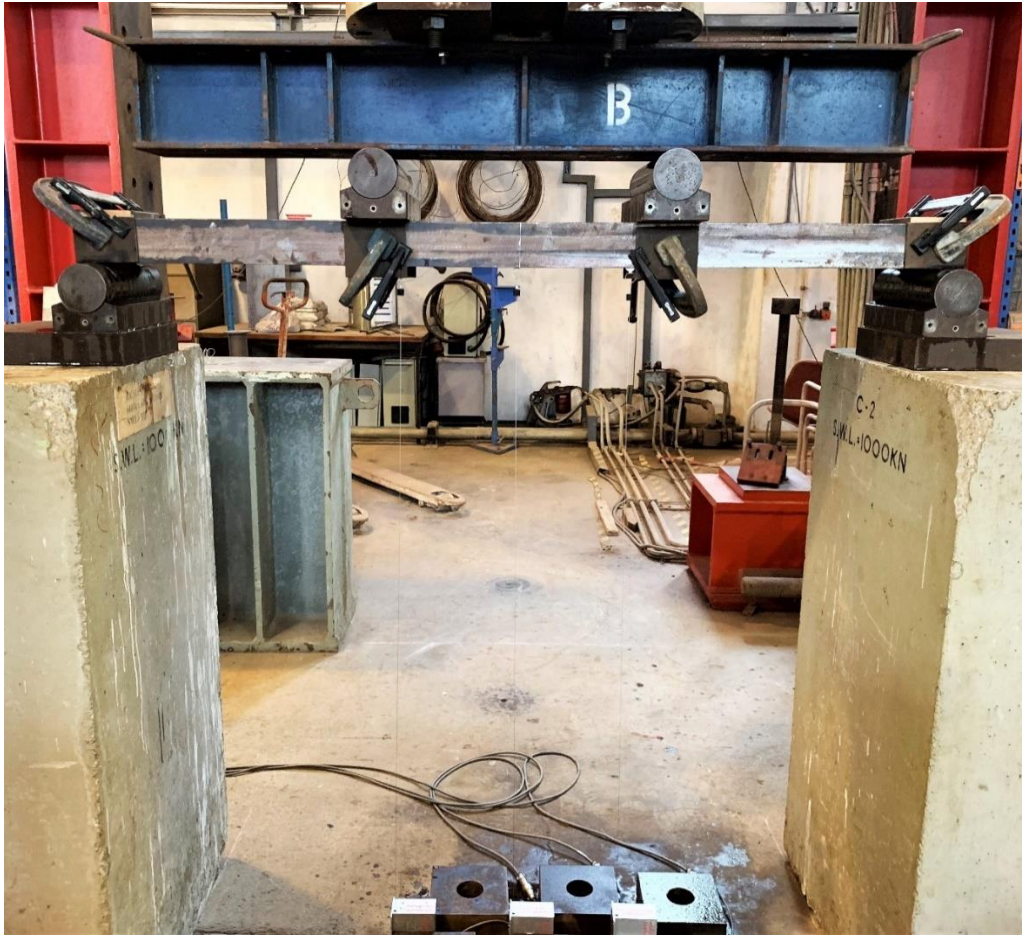
Fig. 4. Minor-axis four-point bending test setup.
