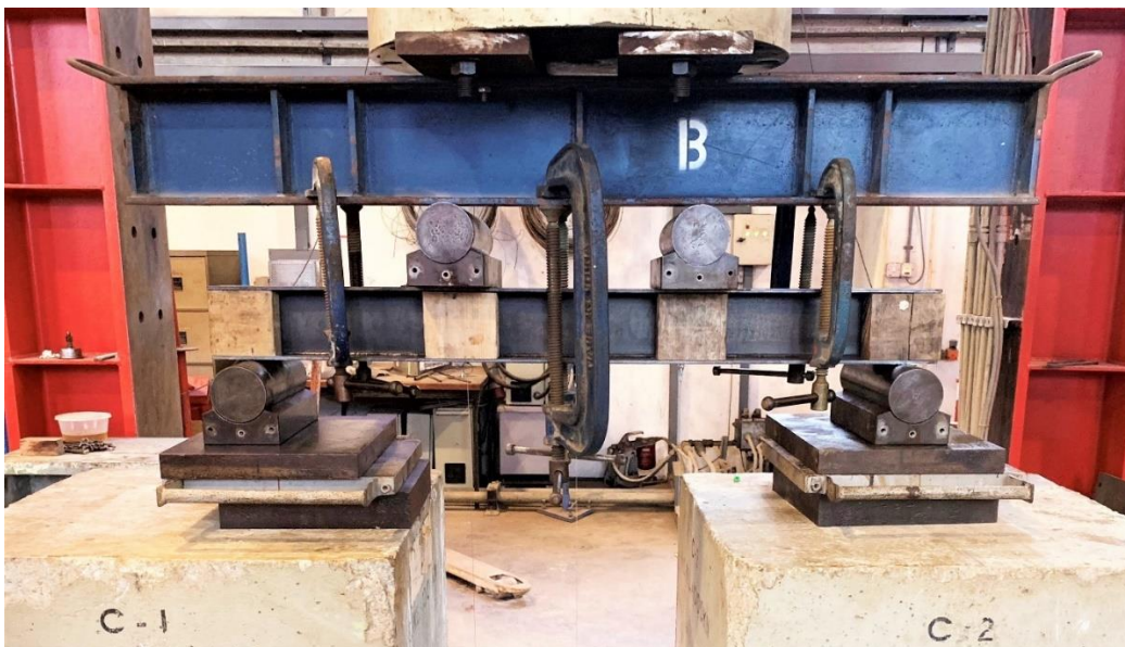
Fig. 5. Major-axis four-point bending test setup.
