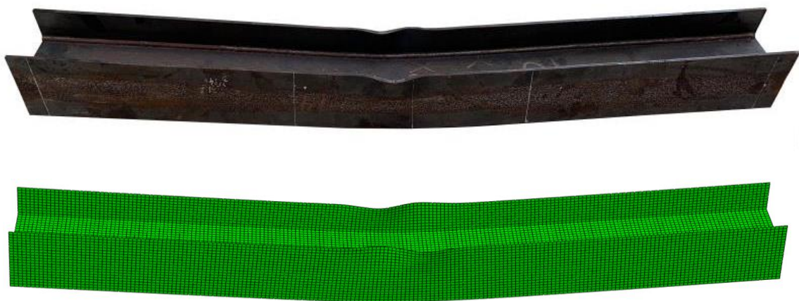
Fig. 7. Test and FE failure modes for beam specimen I-100×100×5-MI in minor-axis bending.
