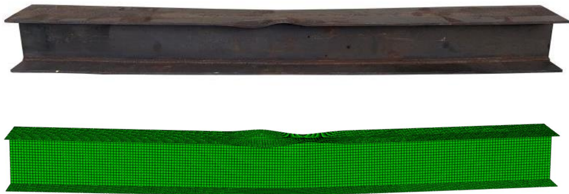
Fig. 6. Test and FE failure modes for beam specimen I-100×100×5-MA in major-axis bending.
