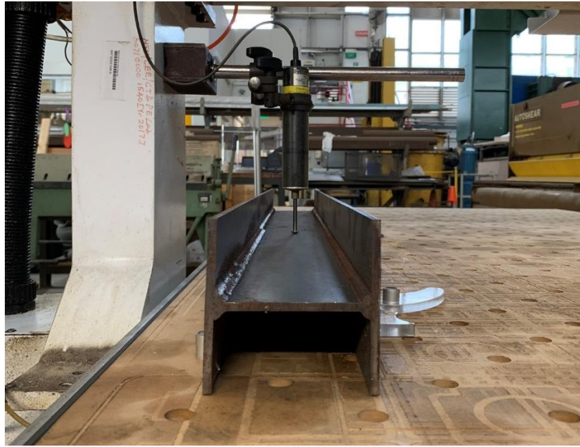
Fig. 3. Test rig for initial local geometric imperfection measurements.
