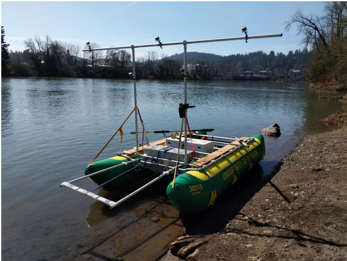
Figure 4: Photo of the raft with the W shaped camera array. The top bar is the base for three cameras, and the two vertical poles are the base for the two remaining cameras. The fiberglass poles extending behind the boat hold a meter-long scale bar used to test the scale of resulting water surface DEMs.
