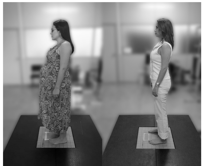
Figure 1. Illustration of a typical participant under force platform for balance measurement (BIOMECH 400). Note: Static balance experimental task conditions: two-legged stance with eyes open and with eyes closed. 50x42mm (300x300 DPI).
