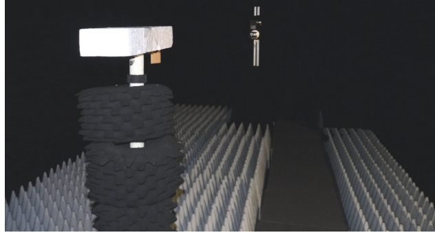
FIGURE 8: Measurement of far-field diagrams in anechoic chamber.
