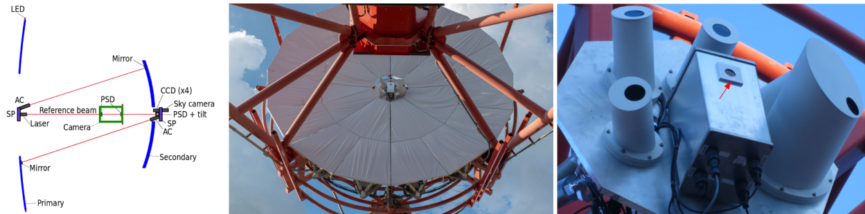
Figure 6.8: The global alignment system of the pSCT. Left: a schematic representation of the GAS. Middle: the secondary mirror dish with the optical table in the center. The mirror panels are covered with a protective white film that was in place during transportation, installation and alignment of the mirrors. Right: a closeup of the secondary optical table. The laser spot used to monitor the optical axis alignment is highlighted with a red arrow right below the window to the PSD. The watertight cylindrical white enclosures house the CCD cameras and the autocollimator.
