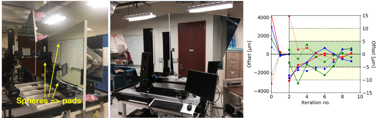
Figure 6.7: MPM calibration. Left : a P1-P2 edge is being calibrated. The half-spheres used to measure the exact position of a mirror panel are highlighted with yellow arrows. The spheres are temporarily fixed to the same exact reference points that were used to glue the Stewart platform attachment pads. The coordinate measuring machine and its probe can be seen on the left. Pink plastic bags cover the calibrated MPES for protection during transportation. Middle : a calibrated P1-P1 edge. Note the continuity of the aligned surface. Right : the convergence of edge misalignment in a laboratory setup. The plot shows readings from a triad of MPES along a P1-P1 edge (as in Figure 6.6, right) during an MPM alignment convergence test. Solid (dotted) lines represent the offset from the target position in the x ( y ) local coordinate system of MPES. The vertical line marks the change of scale along the y axis. For this test, the initial edge misalignment was 4 mm.
