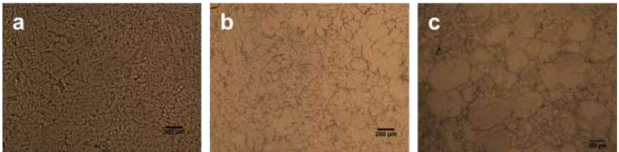
Fig. 3. Morphological transition of Sn-20Bi alloy microstructure from (a) dendritic to (c) globular via (b) rosette. (a) is without shear and cast at 230 °C, (b) sheared less than 1 minute at 205 °C, and (c) sheared for 5 minute (total) at 195 °C.
