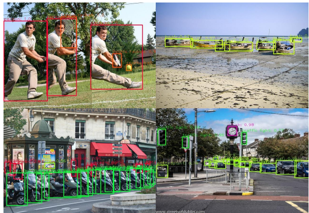
Figure 6. Detection results of the proposed HSD on the COCO minival set. It can be seen that the proposed HSD has a good detection performance on small-scale objects and occluded objects.
