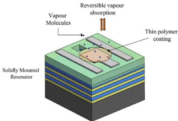
Fig. 2. Schematic of polymer-coated SMR for VOC detection.
