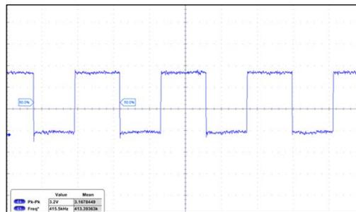
Fig. 3. Typical output of the complete system. Frequency count is performed by the microcontroller.
