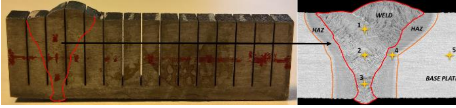
Figure 4: Comb-like reference sample used to determine stress-free lattice spacing and the neutron diffraction measurement locations on the reference sample.
