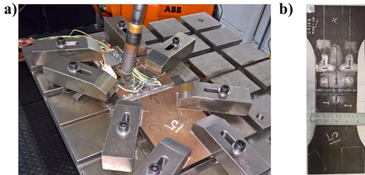
Figure 1: Specimen manufacturing a) Welding set-up with thermocouples and strain gauges b) Final specimen after EDM cut.
